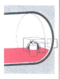
flexibility. These controls are engineered to be easily adaptable to a wide range of conditions. For instance, over a period of time the amount of oil, gas and water in the wellstream may change. The controls can be adjusted to vary the level at which liquids are dumped, up to the height of the permanent gas treatment components, This allows flexibility for liquid-gas ratios other than originally specified.
