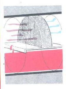
esces into large droplets which fall to bottom of tank. With the knitted wire mesh mist extractor, BS&B is able to limit liquid carryover to 1/10 gallon per million cubic feet of gas on all particles 10 microns and larger. Where there is slight foaming action, a second extractor is installed behind the first. (For serious foam problems check BS&B Foam Separators.)
