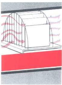
Gas enters the vanes, an area of controlled, one-direction movement. This reduces turbulence. And the reduction in turbulence allows the highest efficiency in recovery of liquids. This is because liquids tend to fall out naturally, through gravity, when the gas stream is in a non-turbulent state.
