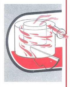
to the bottom. Gases escape through an opening in the top of the deflector. Liquids are rushed to the liquid area quickly, reducing reentrainment tendencies.
