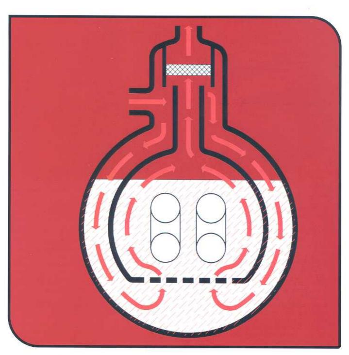
Featuring the H.U.T. Treater with up-flow in both the firebox section and the filter section for greater efficiency, longer firebox life, less maintenance.
