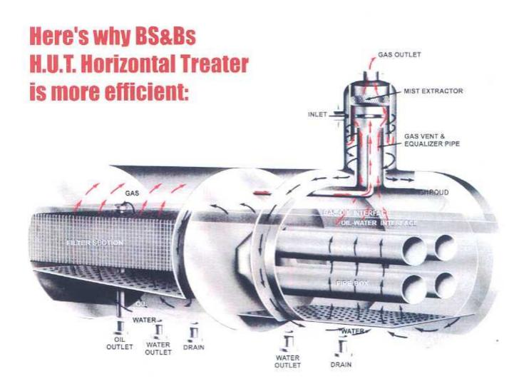
The BS&B H.U.T. Treater borrows the best features of the dependable vertical treater, and combines them with the high capacities of the horizontal treater.
